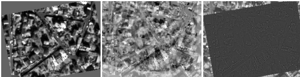
Figure 9.12: Resampled moving image (left). Differences between the fixed and moving images, before (center) and after (right) registration with the CenteredRigid2D transform.
