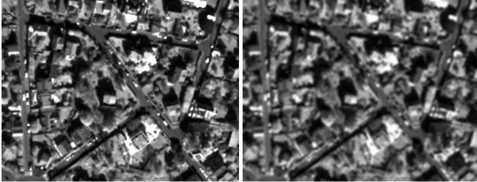
Figure 8.24: Result of applying the otb::MarkovRandomFieldFilter to an extract from a PAN Quickbird image for restoration. From left to right : original image, restaured image with edge preservation.
