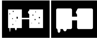
Figure 25.9: The effects of morphological operations on a binary image using a circular structuring element of size 4. Left: original image. Right: dilation.
