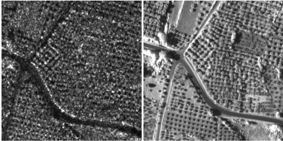
Figure 9.7: A SAR image (fixed image) and an aerial photograph (moving image) are provided as input to the registration method.
