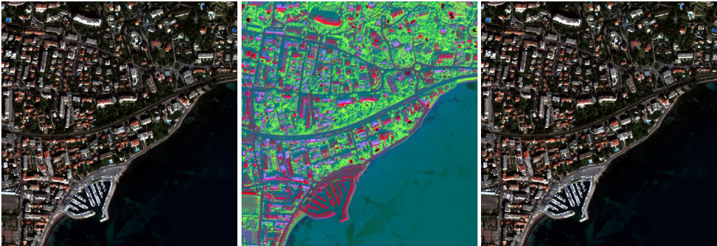
Figure 18.1: Result of applying the otb::PCAImageFilter to an image. From left to right: original image, color composition with first three principal components and output of the inverse mode (the input RGB image).
