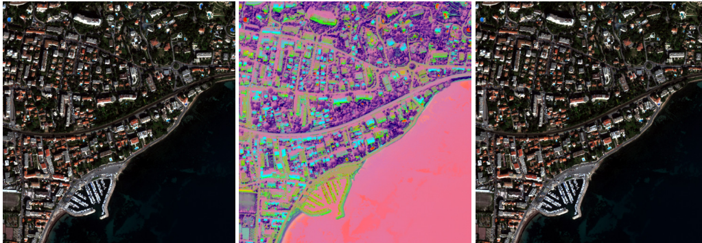
Figure 18.3: Result of applying the otb::MNFImageFilter to an image. From left to right: original image, color composition with first three principal components and output of the inverse mode (the input RGB image).
