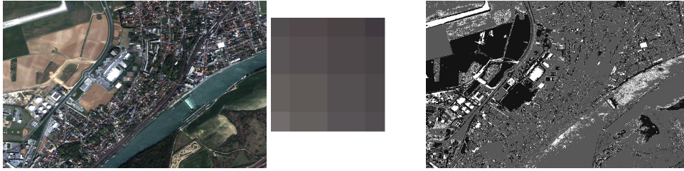
Figure 19.5: Result of the SOM learning. Left: RGB image. Center: SOM. Right: Classified Image
