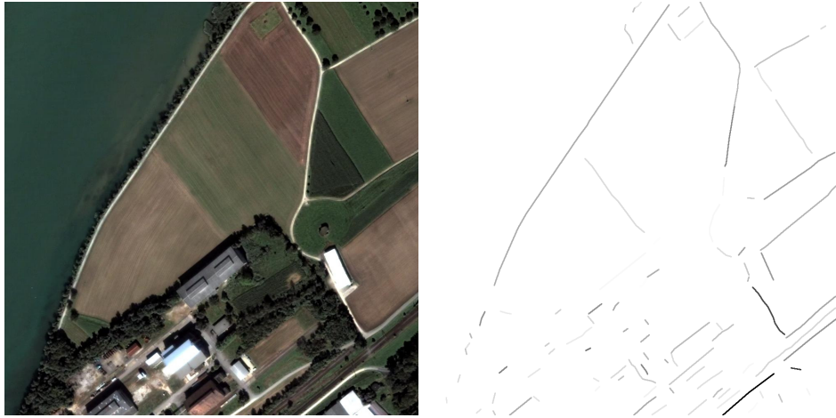
Figure 14.12: Result of applying the otb::RoadExtractionFilter to a fusionned Quickbird image. From left to right : original image, extracted road with their likelihood values (color are inverted for display).
