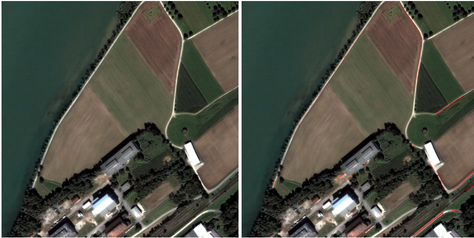
Figure 14.14: Result of applying the road extraction by steps pipeline to a fusioned Quickbird image. From left to right : original image, extracted road with their Likelihood values.
