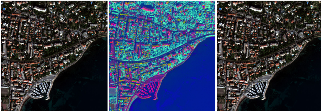
Figure 18.2: Result of applying the otb::NAPCAImageFilter to an image. From left to right: original image, color composition with first three principal components and output of the inverse mode (the input RGB image).
