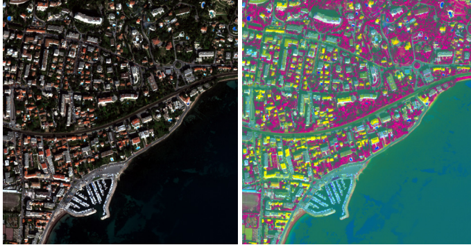
Figure 18.5: Results of the Maximum Autocorrelation Factor algorithm applied to a 8 bands Worldview2 image (3 first components).
