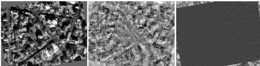
Figure 9.10: Resampled moving image (left). Differences between the fixed and moving images, before (center) and after (right) registration using the CenteredRigid2D transform.
