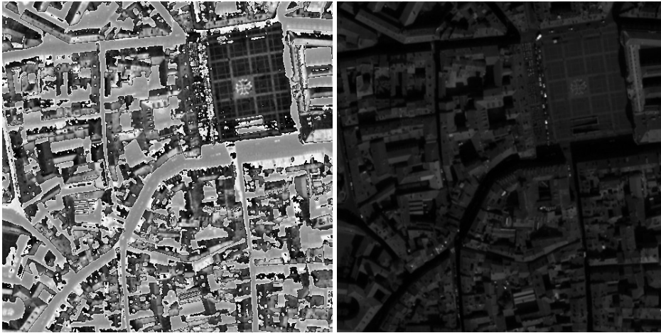
Figure 23.1: On the left, the image obtained by truncated pixel values at the dynamic acceptable for a png file (between 0 and 255). On the right, the same image with a proper rescaling
