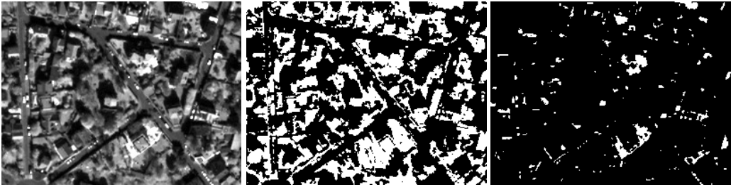
Figure 26.2: Using ImageAdaptor to perform a simple image computation. An ImageAdaptor is used to perform binary thresholding on the input image on the left. The center image was created using a threshold of 100, while the image on the right corresponds to a threshold of 200.
