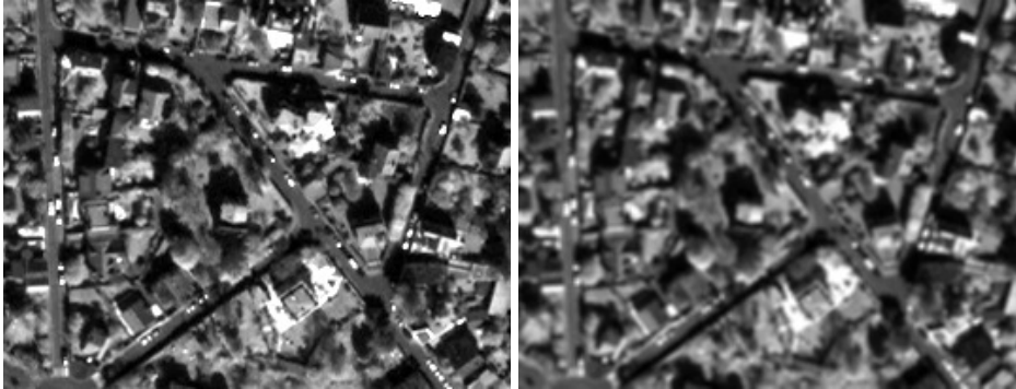
Figure 8.14: Effect of the MeanImageFilter.
