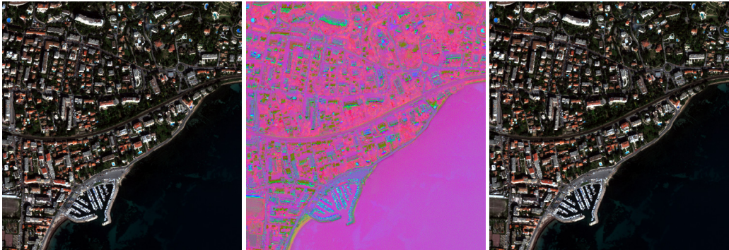
Figure 18.4: Result of applying the otb::FastICAImageFilter to an image. From left to right: original image, color composition with first three principal components and output of the inverse mode (the input RGB image).
