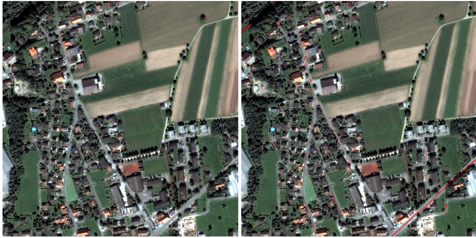
Figure 14.15: Result of applying the road extraction by steps pipeline to a fusionned Quickbird image. From left to right : original image, extracted road with their Likelihood values.
