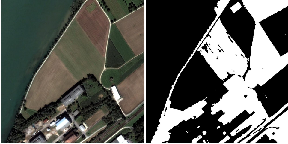
Figure 8.6: From left to right: Original image, thresholded NDVI indice.
