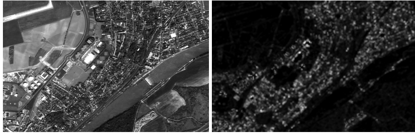
Figure 14.2: Result of applying the otb::ScalarImageToPanTexTextureFilter to an image. From left to right: original image, PanTex feature.
