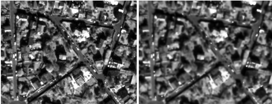
Figure 8.20: Effect of the GradientAnisotropicDiffusionImageFilter.
