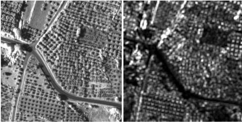
Figure 14.1: Result of applying the otb::ScalarImageToTexturesFilter to an image. From left to right : original image, contrast.
