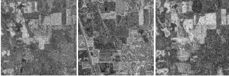
Figure 22.6: Result of applying the otb::VcaImageFilter and otb::UnConstrainedLeastSquareImageFilter to an image. From left to right and top to bottom: first abundance map band, second abundance map band, third abundance map band.
