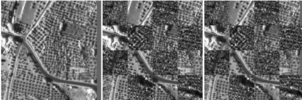
Figure 9.8: Mapped moving image (left) and composition of fixed and moving images before (center) and after (right) registration.
