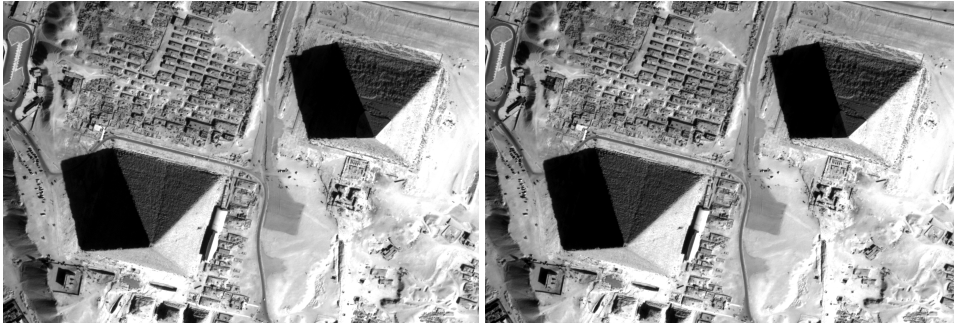
Figure 4.17: Extract of resample image1 and image2 in epipolar geometry over Pyramids of Cheops. ©CNES 2012
