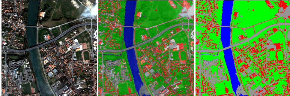
Figure 4.12: From left to right: Original image, result image with fusion (with monteverdi viewer) of original image and fancy classification and input image with fancy color classification from labeled image.
